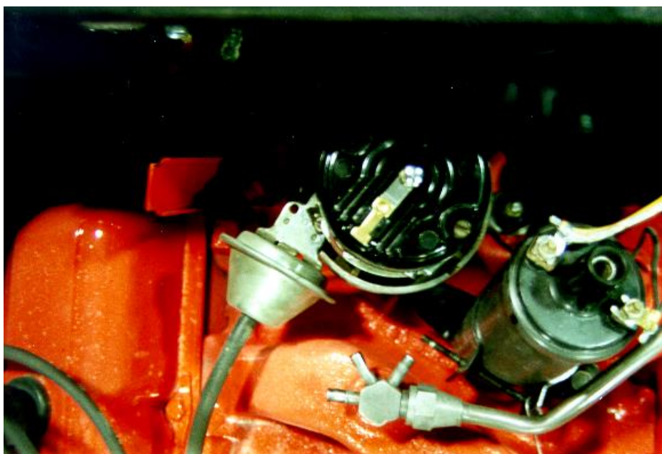
Figure 1: Distributor & Rotor Correctly Installed at #1 Firing Position
