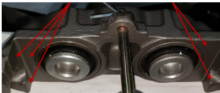
Fig. #2. RF Caliper side. Red arrows show machined area's around the pistons.
