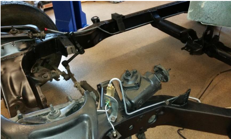
After frame reconditioning and new brake & fuel lines.
