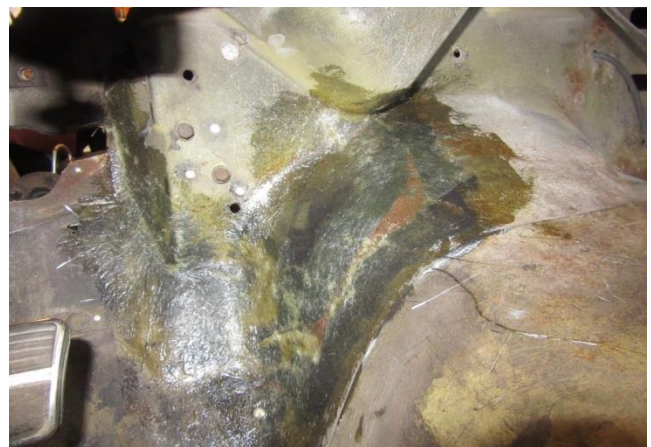
Fiberglass repair and power brake prep.
