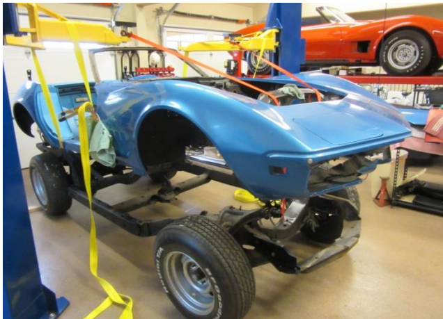
The "Lindee" 2 post body lift method.
